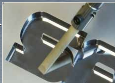
[Finishing] Using wood tip and diamond paste
